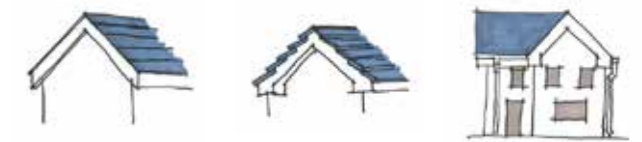
Figure 16.28 Avoid roofs with large overhangs which result in the roof sitting like a 'lid' on the building.
